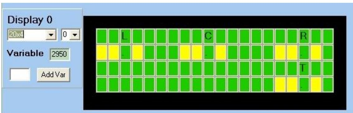
Var 2950 is used as virtual screen selector, if we assign it the value 0, then this fuel screen will show up. Certain positions are given fixed text values, like the L, the C and the R, and the decimal points.
