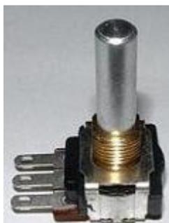
An encoder that is gray type and will work is CTS corporation type 288. A CTS type 288 encoder is available in the [Opencockpits shop](#). Examples of how to program a [gray type encoder in SIOC](#) can be found at the [howto page](#).
